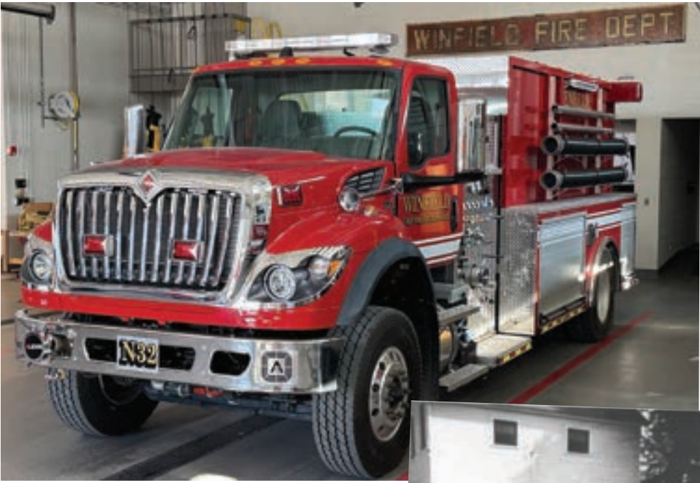
Bottom: Winfield’s first water tender, a 1935 Ford, held 800 gallons of water. Left: Winfield’s newest water tender, a 2025 International Alexis. It can pump 1,250 gallons per minute and can transport 2,000 gallons of water.
